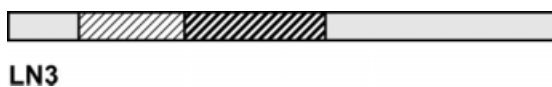
Figure 1 Scheme of the molecular architecture of the styrene-butadiene copolymer LN3 used in this study. This block copolymer is composed of two outer PS blocks (in gray color) which surround two random styrene-butadiene blocks (soft phase, in hatched style).
